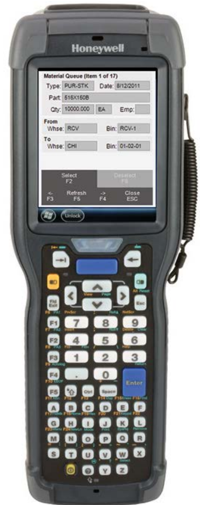
Figure 6.5 Handheld—See improved inventory accuracy with wireless device management of inventory functions, such as on-the-fly adjustments and viewing the material queue.
